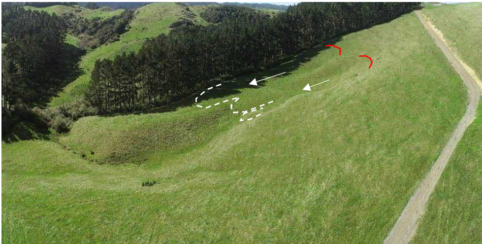
Photograph 2: Oblique aerial view of the Stage 1 western gully. Historic headscarp [red] and debris run out [white].
